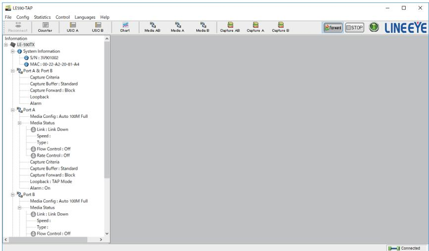
Capture packets of target line using the LE590-TAP (TAP mode).
